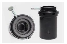
GRIP-TIGHT™ Nuts can be torqued and loosened with common impact guns and wrenches. The patent pending washer profile includes a special geometry for rotationally coupling to the HYTORC reaction socket. This washer acts as a coaxial reaction point, thereby eliminating pinch points and removing undesirable side loads. These benefits make it feasible to upgrade to cordless digital tooling systems while increasing the efficiency, quality and safety of wheel nut installations.
